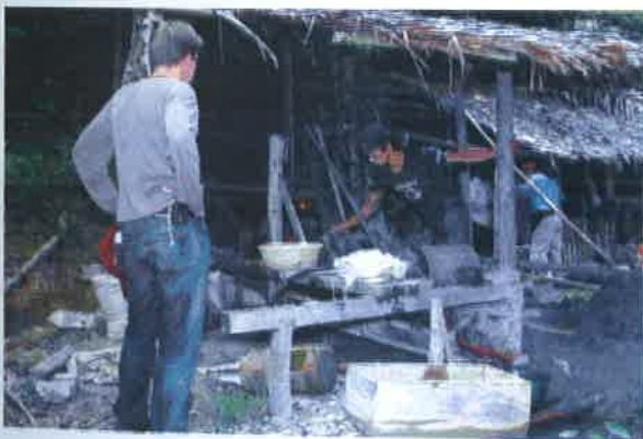
Figure 5. "Gelundung" or "teromol" facilitated for pulverizing crushed ore to become amalgam.
