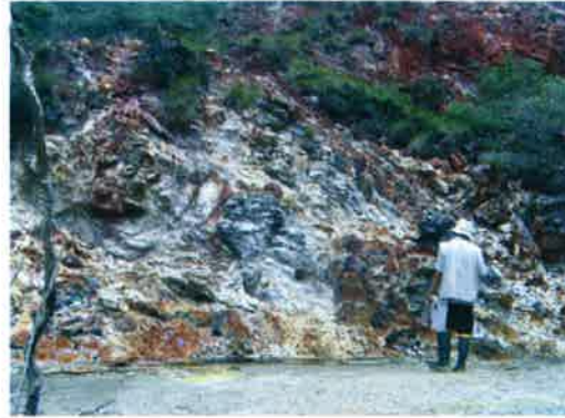
25d. AP. 99,2°C, tanah panas 82°C, pH 8.82 debit 0,2 lt/det Alterasi: illite, kaolinite
