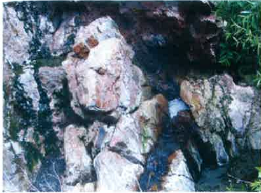
25f. AP. 101.3°C, debit 0,5 lt/det, tanah panas 86°C, sinter silika Alterasi: illite, alunite
