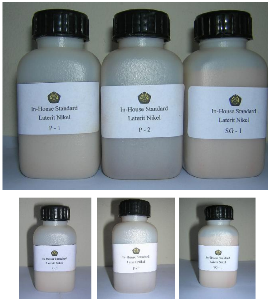
Gambar 15. Hasil pengemasan In-House Standard contoh laterit nikel
